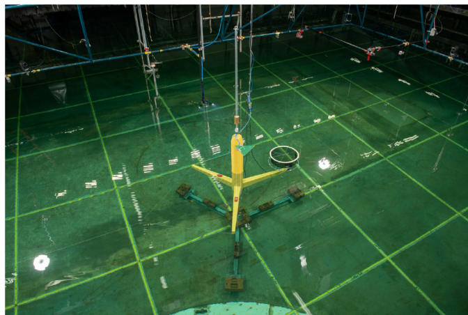
Model test of fish cage and TLP in MARIN wind, wave and current basin.
