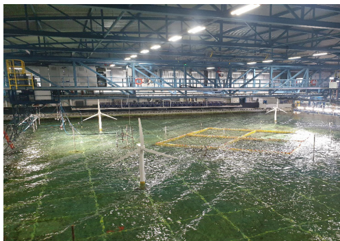
Figure 1: Concept I: Closed net pen within offshore wind park
