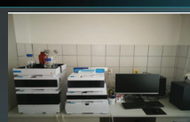
High Performance Liquid Chromatography (HPLC)
