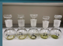
Extraction of total lipids by the Folch method
