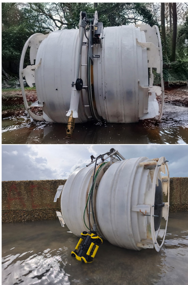
MAR equipped with a multiparametric probe and with an underwater ROV
