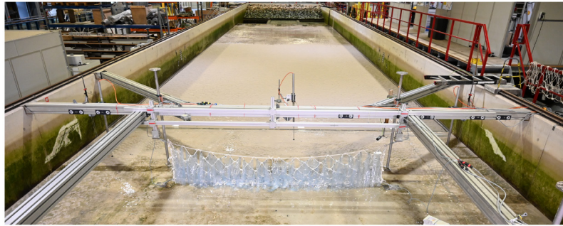
Figure 1. Seaweed net test setup in 90 degree orientation (wave/current perpendicular to the net)
